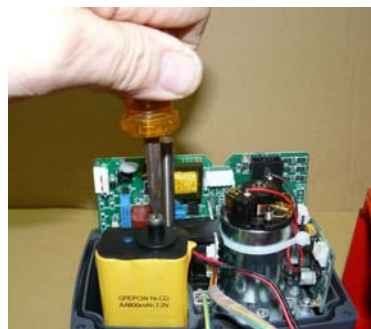
Photos showing the alternate location for the battery in the J3-L Series actuators, models 20, 35 & 55.
